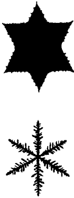
Figure 1. Patterns of viscous fingers for mobility ratio M = 5 (top) and M = 1000 (bottom), obtained on a triangular network.
